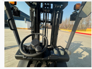
Wide field of view back pipe mast
