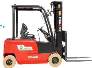
III 1.6-2t four wheels dual driving motors counterbalance electric forklift
