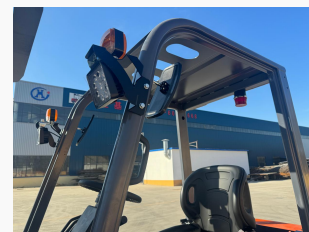
Energy saving LED lights
