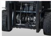
imported German SCHABMULLER double drive motor
