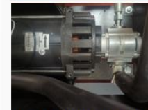
KDS lifting motor and Eckerle lifting pump
